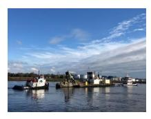
The dredge *Borinquen* has arrived in Topsail Creek and started placing sand on the beach on December 1<sup>st.</sup> The sand is being placed on the beach south of the Drum Avenue access to start the project. Once that work is complete, the pipes will be relocated, and the beach nourishment process will move north. Periodically the *Borinquen* will move and pumping activity will stop for a
